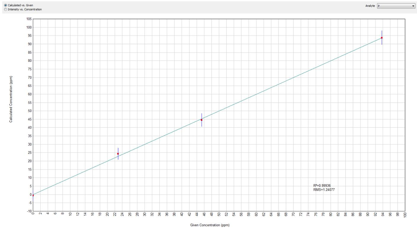
Figure 2b : Calculated versus given concentrations in the case of zinc (Zn)
