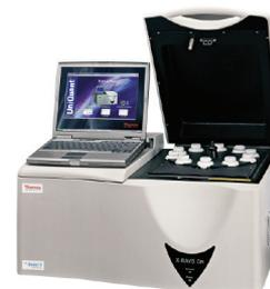
The Thermo Scientific ARL QUANT'X is equipped with a Peltier-cooled Si(Li) detector of 3.5mm thickness. This thickness ensures high stopping power for higher energy X-rays produced by heavier elements like precious metals. Table 1 shows the detection limits obtained for Rh, Pd and Pt in a typical ACC matrix.
