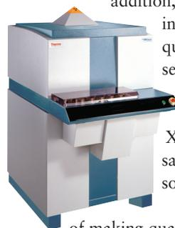
addition, an XRF goniometer can be installed for qualitative or semi-quantitative investigations and sequential analysis of any of 83 elements of the periodic table. Hence, this instrument performs XRF and XRD analysis on the same sample with the same hardware and software environment.
