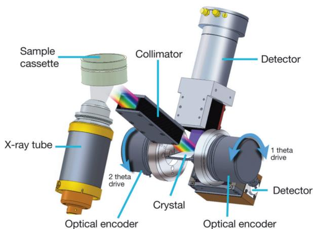
**Figure 1.** The heart of the Thermo Scientific ARL OPTIM'X WDXRF spectrometer.
